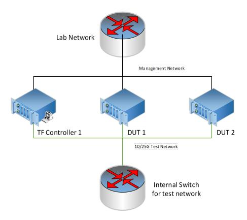
Generally, the physical topology has 2 networks, 1 network is for management and the other network is for test.
